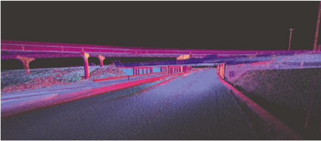
LiDAR scan data (top) provide input for 3-D modeling and rendering (bottom), which was created in Autodesk InfraWorks.
